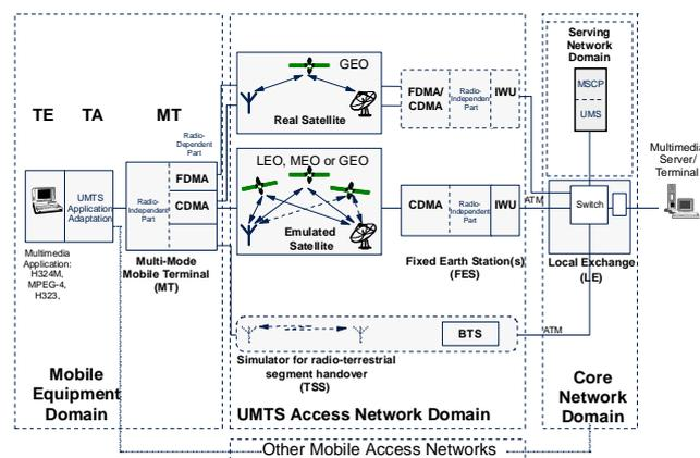
Figure 1: SUMO testbed
