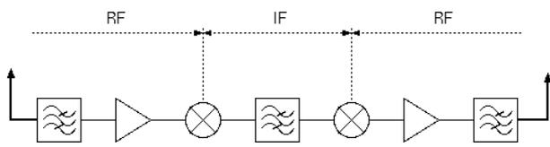
Figure 13: Architecture for unidirectional simple repeater
