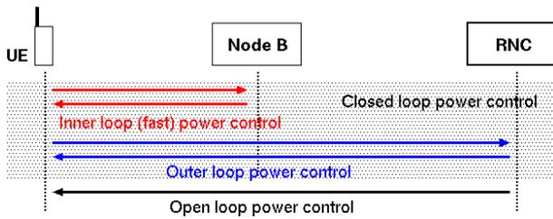
Figure 9: W-CDMA power control mechanisms
