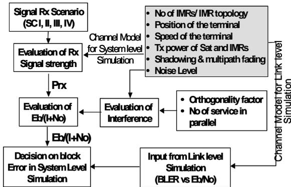
Figure 4: Interface between the link/ system level
