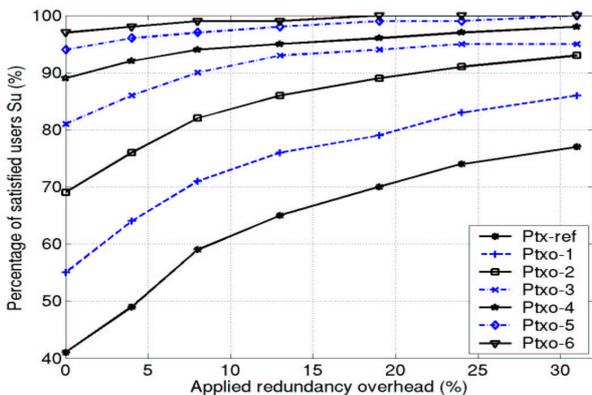
Figure 7:  $S_u$  variation with redundancy overhead for different transmit power levels; RMTP layer PLR 5%
