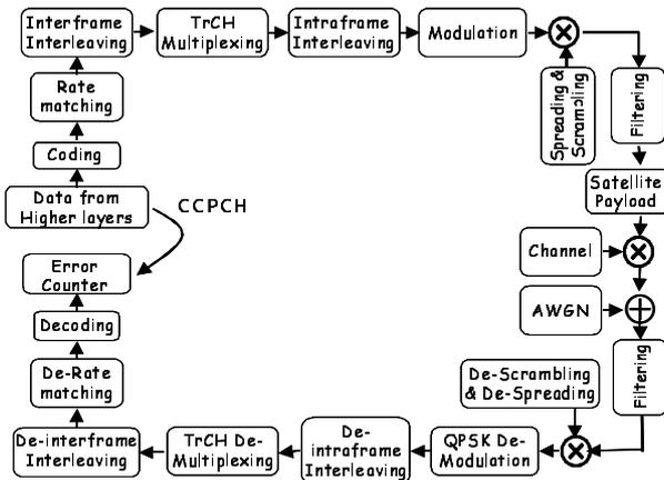
Figure 2: Physical layer Simulator
