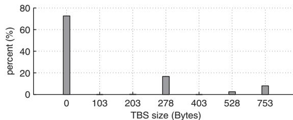
Figure 8. Transport block set size distribution for FACH 4 at S-CCPCH
