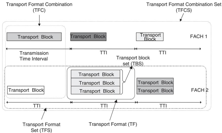
Figure 3. Example of data exchange between MAC and the physical layer when two FACHs are multiplexed.
