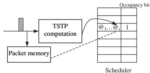
Figure 5. Virtual spacing: arrival of a packet.
