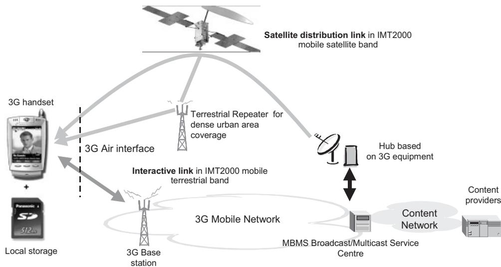
Figure 1. SDMB system and position with respect to the terrestrial 3G mobile networks.
