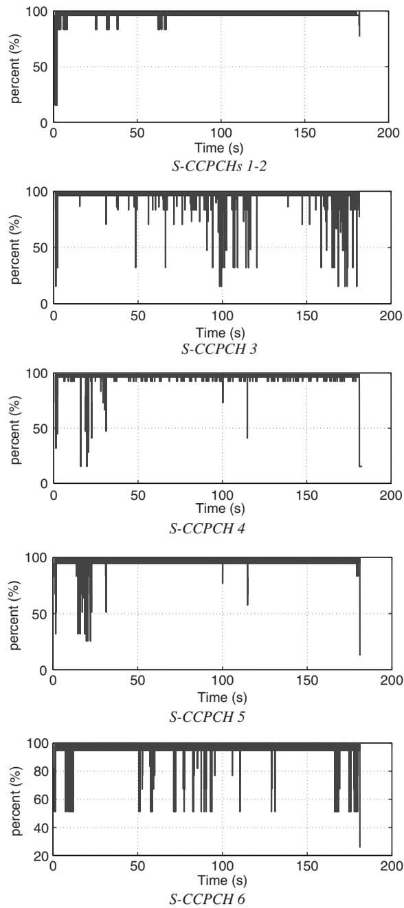
Figure 10. Per S-CCPCH utilization versus time—MLPQ-based scheme, bin-packing.
