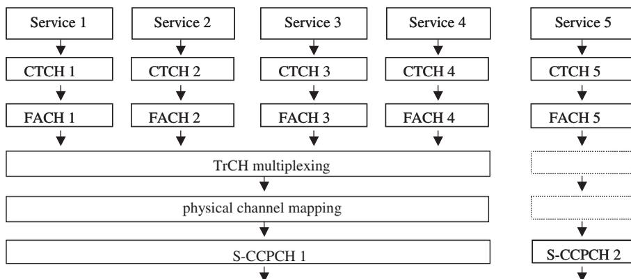
Figure 2. The common downlink WCDMA channels used for MBMS data transfer over the satellite radio interface.
