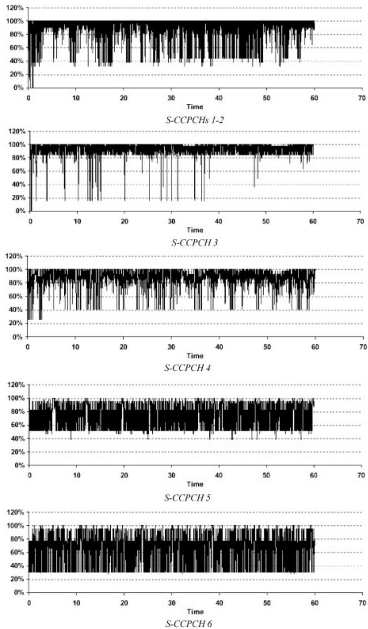
Figure 12. Per S-CCPCH utilization versus time—WFQ-based scheme, bin-packing.
